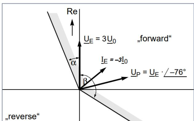
Our algorithm developed for use with calculated zero sequence current. But if you decide to use recorded zero sequence current you have to clearly understand what current you will use and how this switch can be used. For example, Siemens relays records current named as **IE**. If you check the manual, you'll see that this current is equal to **-3I0** and if you link this current to the **3I0** input of the impedance calculator you need to turn **Inversion** switch.
