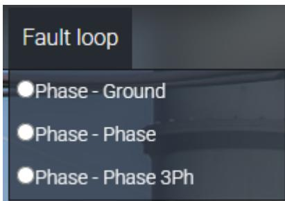
**Fault loop** menu is used to select an appropriate short circuit loop and it determines the calculation algorithm in the impedance calculator and characteristics of distance zones shown (they may differ for single and multiphase short circuits).
