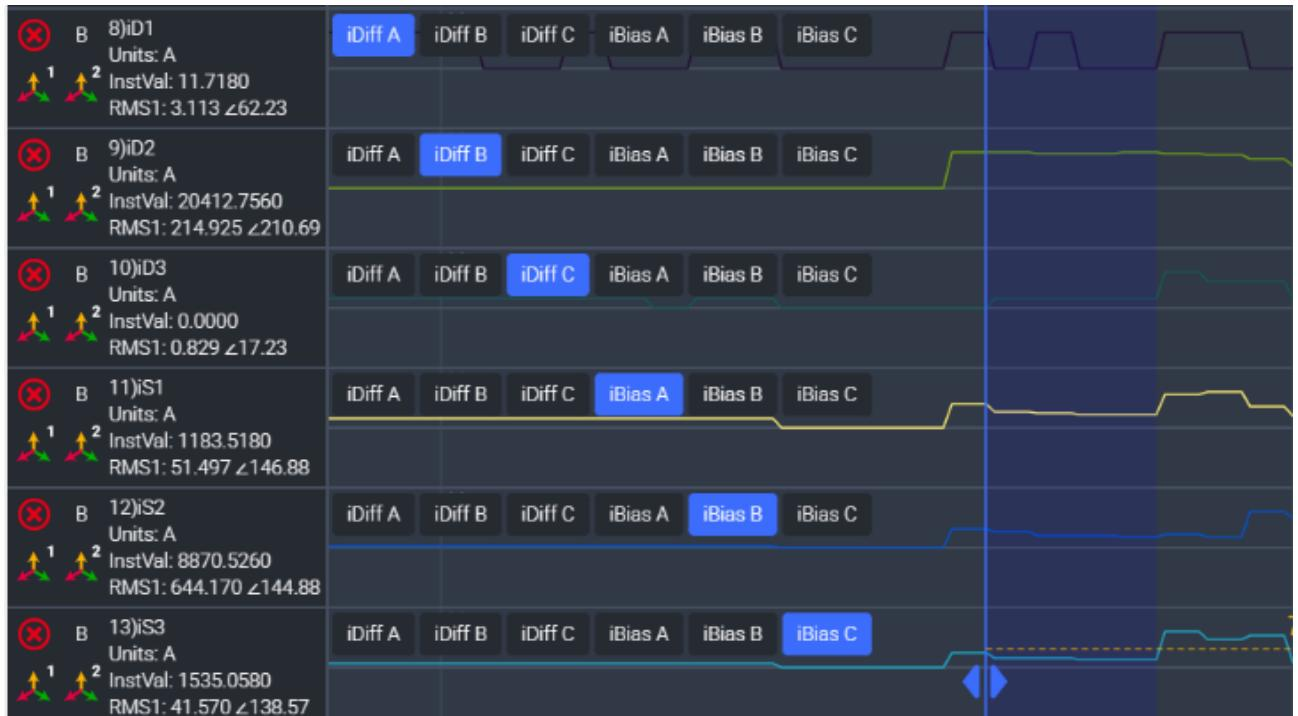
Example with phase **B** to ground short circuit on 330 kV line protected by 7SD522 relay visualized with **3Diff/3Bias linker** and **7SDxxx** element
