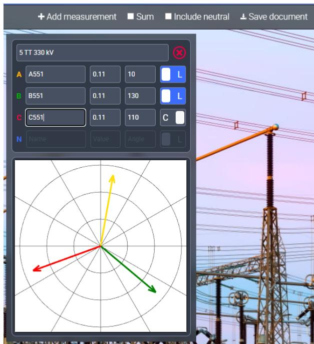
This page is used to visualize phasors (vectors) measured during CT or VT secondary circuits check and save measurements to a report.
