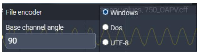
Option **File encoder** allows you to change file encoder from Windows to DOS encoding. This can be useful if you have to deal with old recorders.
