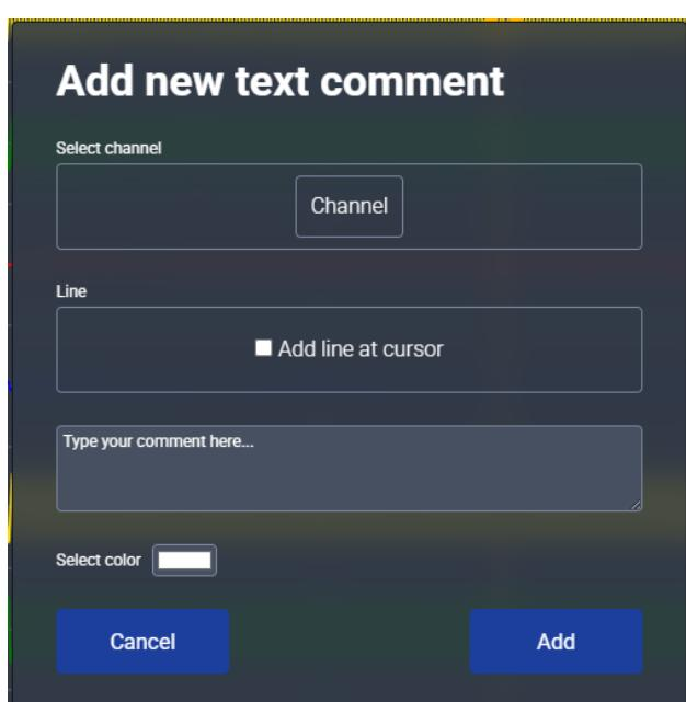
Option **Text comment** prints inserted text on selected analog channel. Also you can add a dash line at the beginning of the comment which goes through all channels.
