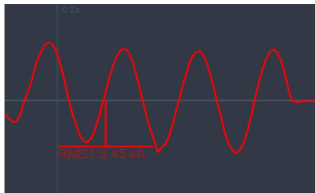
Analog channel with placed mark which contains the first harmonic RMS value. If not any channel selected the mark will be added to the first channel.
