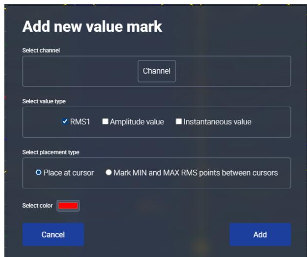
Option **Value mark** is used to add measured value to the analog channel. Firstly, you have to choose a channel for marking, then select value and placement type. By default, red color is used but it is changeable.
