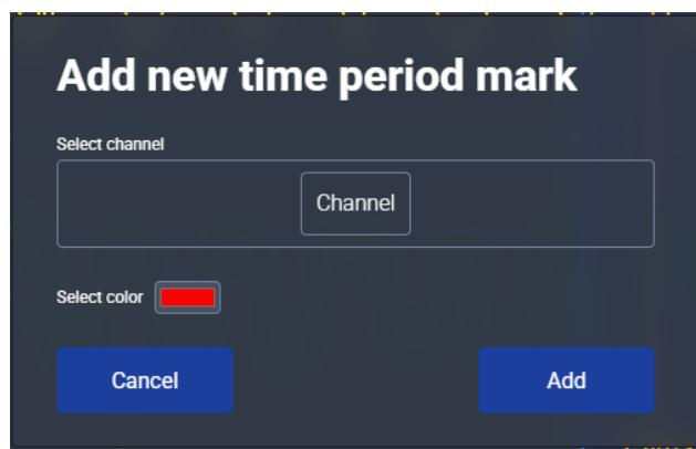
Option **Time period mark** is used to add measured time between cursors (depends on the settings it can be milliseconds, degrees, or cycles).
