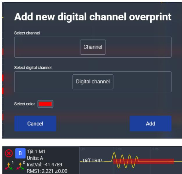
Option **Digital channel overprint** prints selected digital channel on selected analog channel.
